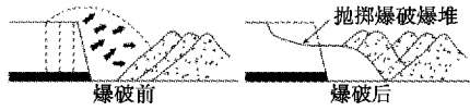
图2 露天煤矿抛掷爆破剥离岩石 Fig.2 Rock stripping by throwing and blasting in open-pit mine
