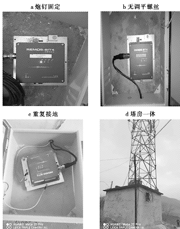
图3 运城站基本二类站烈度计安装问题情况 Fig.3 Installation problems of intensity meters for basic class II stations at Yuncheng Station
